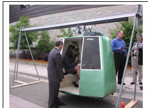
Figure 3. JPod's suspended system
