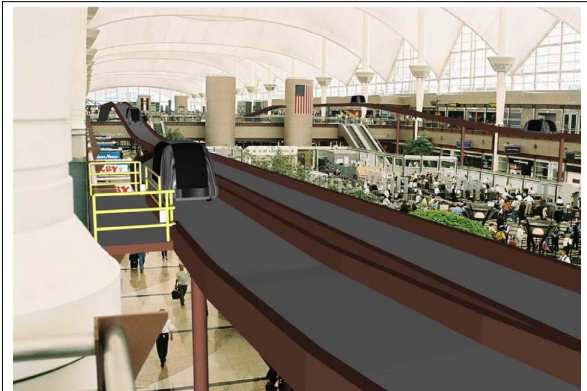
Figure 6. Rendering of a PRT system inside the DIA main terminal. While the system looks large in the foreground, observing the return guideway in the background provides an appreciation of its small scale.
