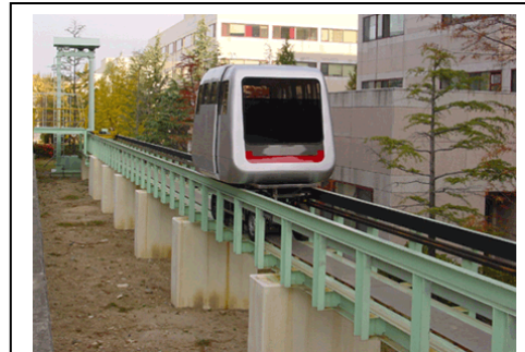
Figure 2. Postech's captive-bogey guideway.
